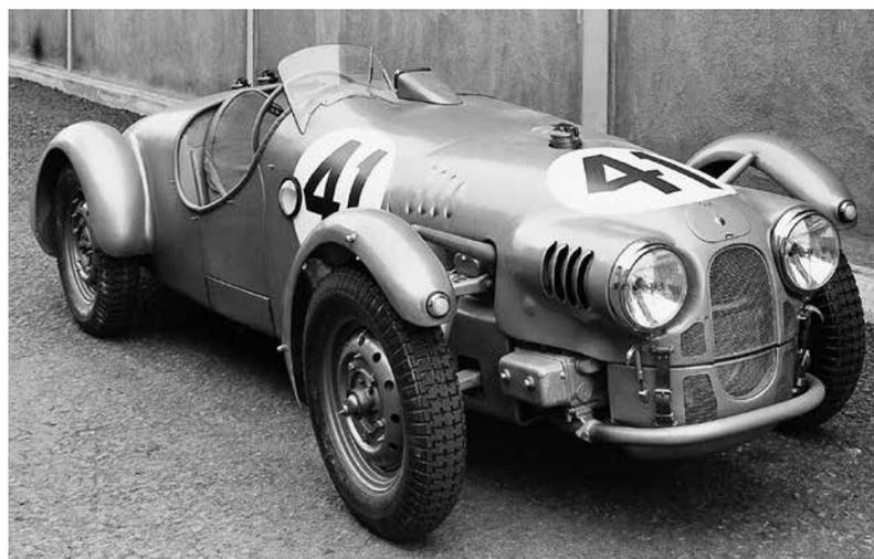
For competition, a lighter, narrower Jupiter with simpler coachwork was proposed and design began soon on the Jupiter type R1; so by early 1951 the sketch above had been produced by Phil Stephenson. The R1 was to be on the Eberhorst chassis, slightly narrowed, as the car would be a 2-seater not a 2/3 seater. So the essential chassis tubing was retained.
